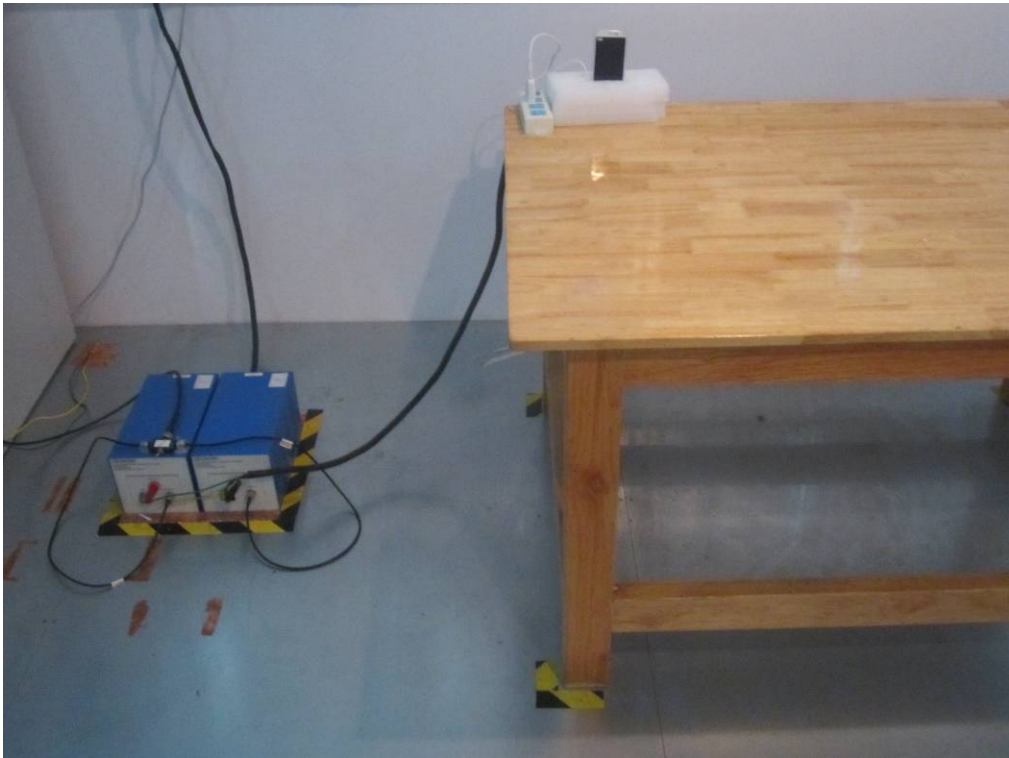
Conducted Emissions Test Setup Front View
