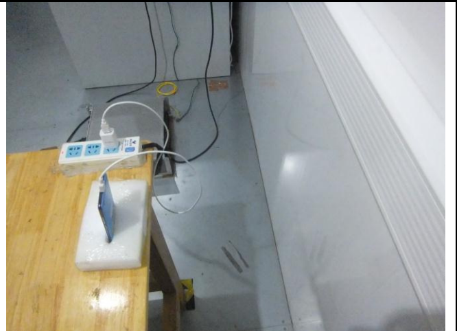
Conducted Emissions Test Setup Side View
