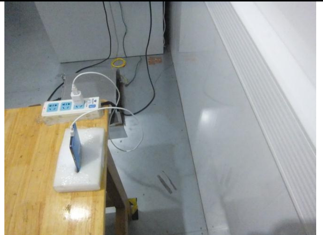
Conducted Emissions Test Setup Side View
