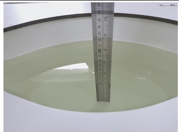
Liquid depth in the body phantom (2450MHz)
