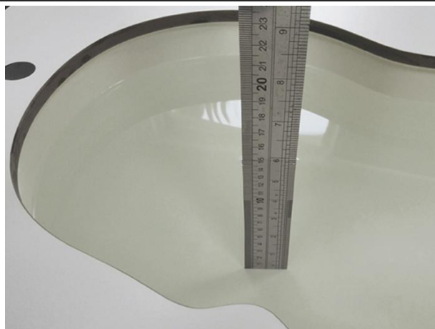
Liquid depth in the head phantom (2450MHz)
