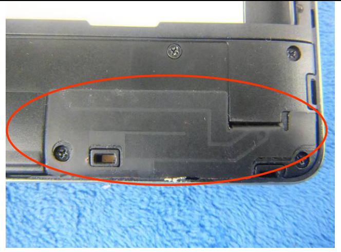
GSM/PCS/UMTS-FDD Antenna View
