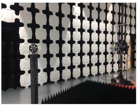
Description: Substitution Antenna for ERP Test
