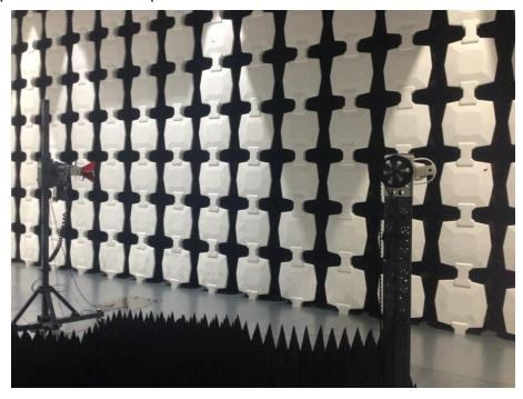
Description: Substitution Antenna for EIRP Test
