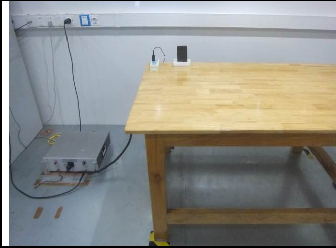
Conducted Emissions Test Setup Front View
