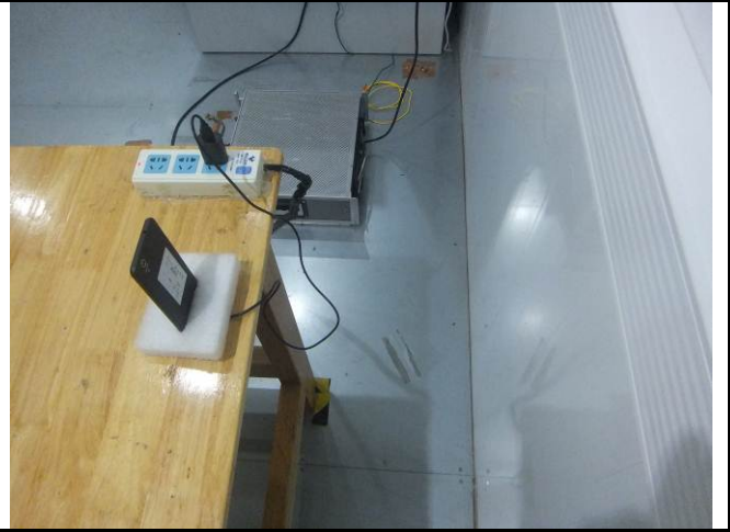
Conducted Emissions Test Setup Side View
