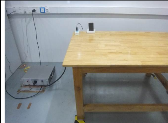
Conducted Emissions Test Setup Front View
