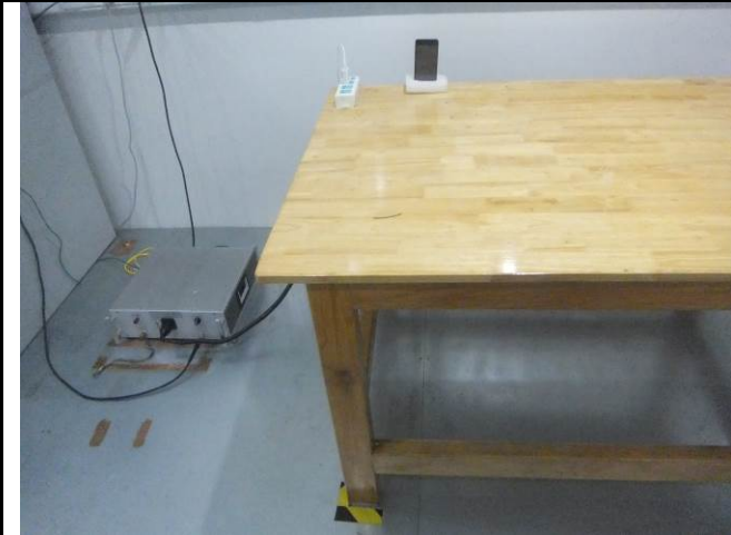
Conducted Emissions Test Setup Front View
