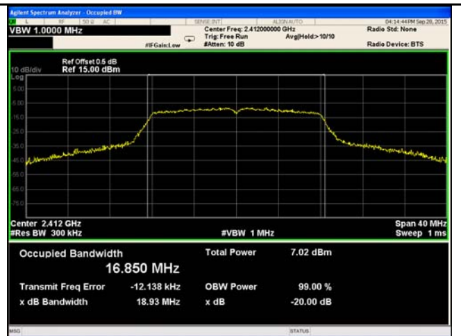
802.11g 20dB Bandwidth - Low CH 2412
