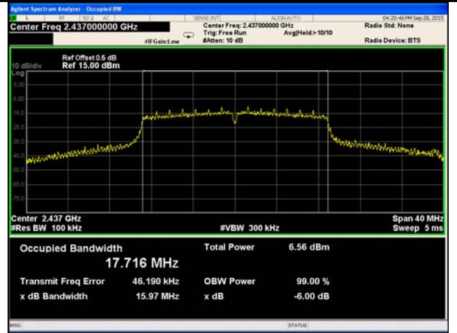
802.11n20 6dB Bandwidth - Mid CH 2437
