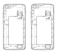
Please insert the SIM card according to the mark on the phone. Make sure that the clipped corner of the SIM card and the metallic contacts are facing the correct direction. Slide the SIM card into the slot until it doesn't move up any further.
