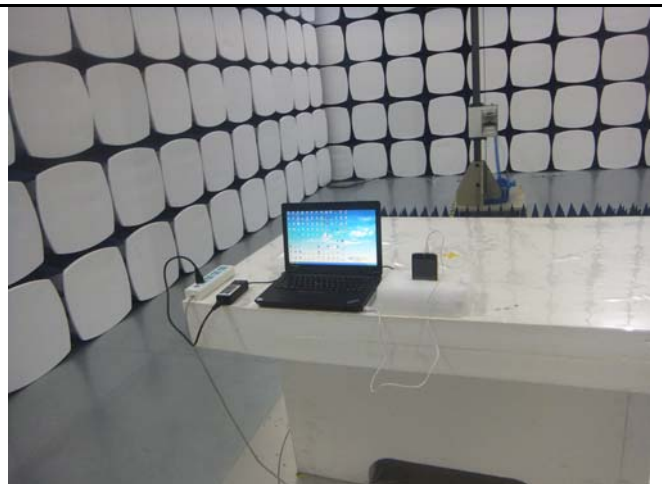
Radiated Spurious Emissions Test Setup Above 1GHz
