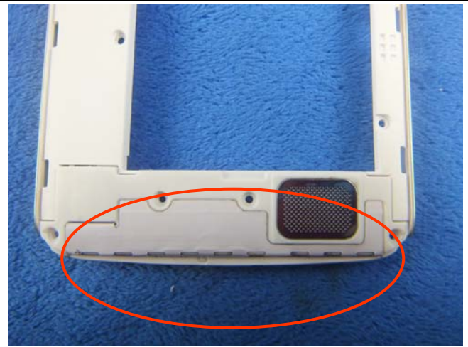
GSM/PCS/UMTS-FDD Antenna View
