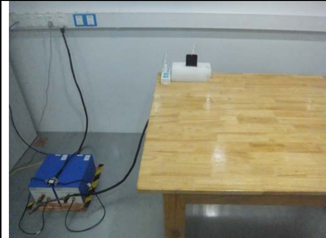
Conducted Emissions Test Setup Front View
