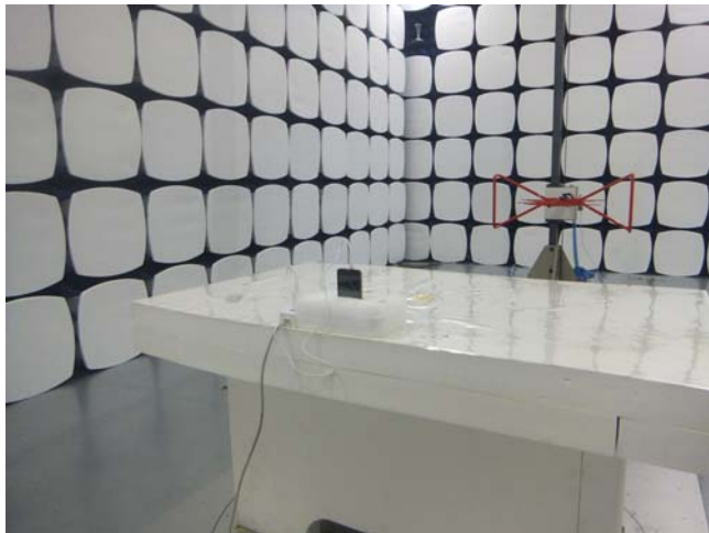
Conducted Emissions Test Setup Front View
