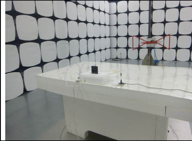
Radiated Spurious Emissions Test Setup Below 1GHz
