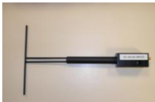
Figure 1 – Satimo COMOSAR Validation Dipole
