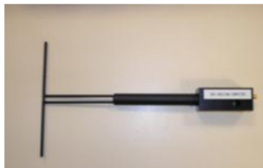
Figure 1 – Satimo COMOSAR Validation Dipole
