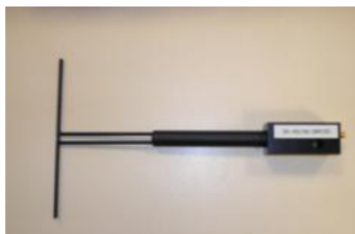
Figure 1 – Satimo COMOSAR Validation Dipole
