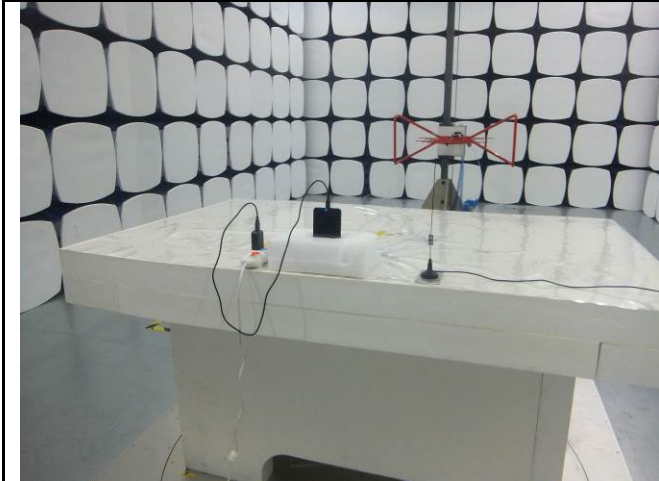
Radiated Spurious Emissions Test Setup Below 1GHz
