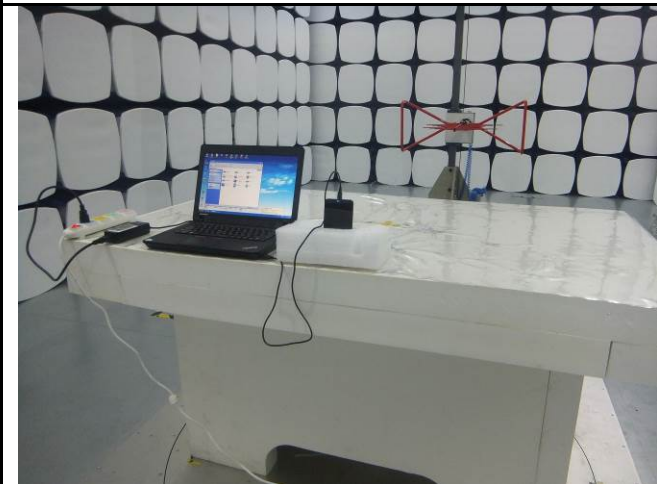
Conducted Emissions Test Setup Front View
