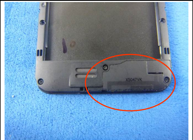
GSM/PCS/UMTS-FDD Antenna View
