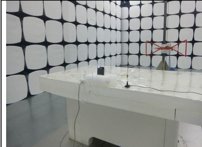
Radiated Spurious Emissions Test Setup Below 1GHz
