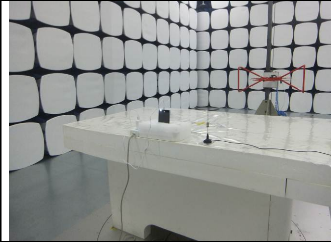
Radiated Spurious Emissions Test Setup Below 1GHz
