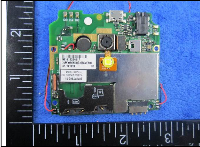
Mainborad With Shielding - Front View
