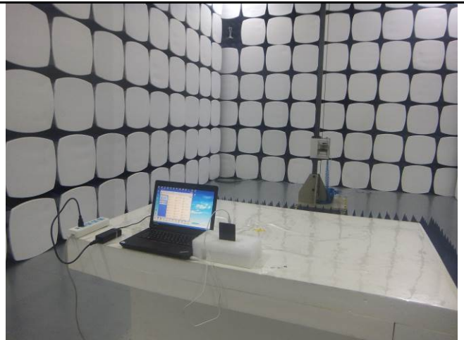
Radiated Spurious Emissions Test Setup Above 1GHz
