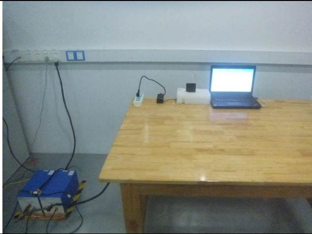
Conducted Emissions Test Setup – Front View
