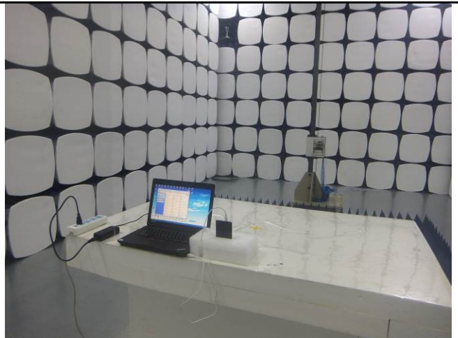
Radiated Spurious Emissions Test Setup Above 1GHz
