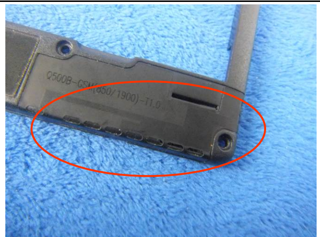
GSM/PCS/UMTS-FDD Antenna View
