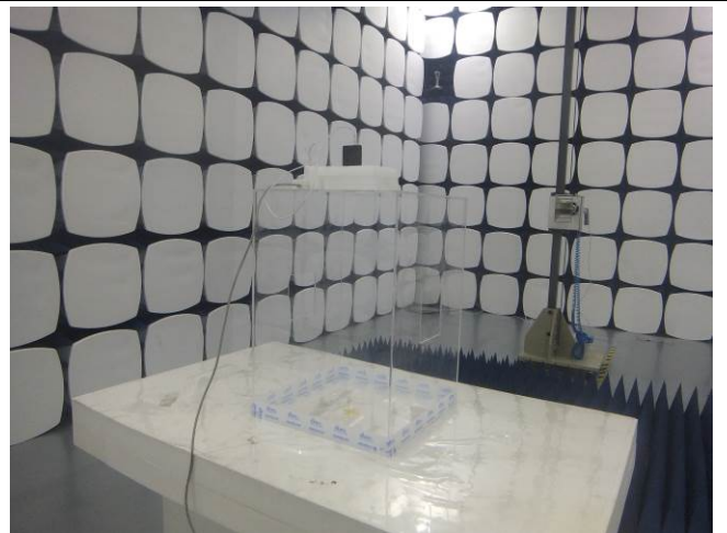
Radiated Spurious Emissions Test Setup Above 1GHz
