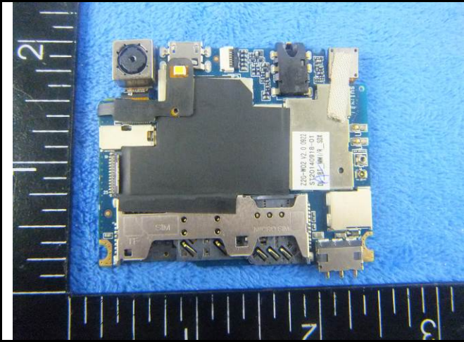
Mainboard With Shielding - Front View
