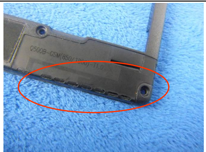
GSM/PCS/UMTS-FDD Antenna View
