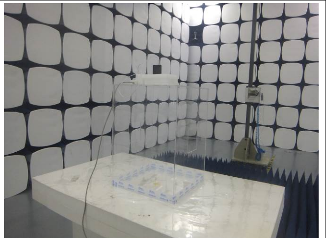
Radiated Spurious Emissions Test Setup Above 1GHz
