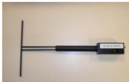
Figure 1 – Satimo COMOSAR Validation Dipole
