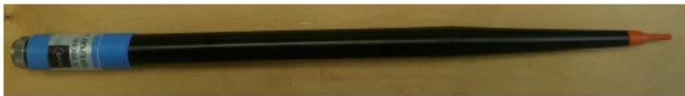
Figure 1 – MVG COMOSAR Dosimetric E field Dipole
