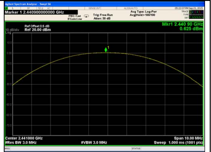
8DPSK Output power - Mid CH 2441
