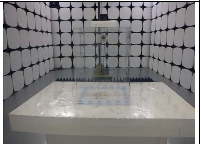
Radiated Spurious Emissions Test Setup Above 1GHz
