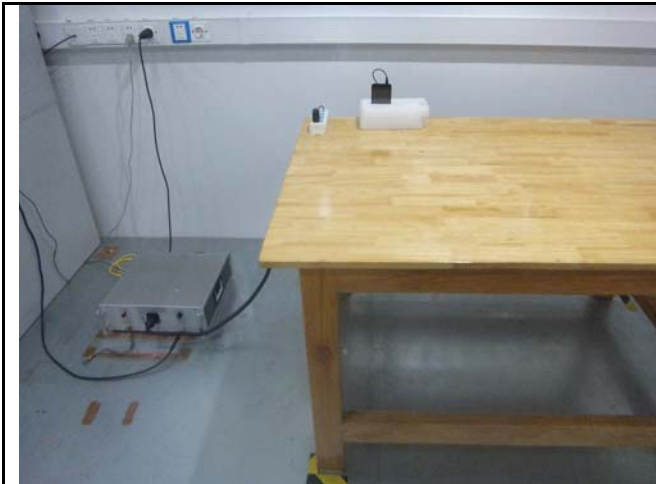
Conducted Emissions Test Setup Front View
