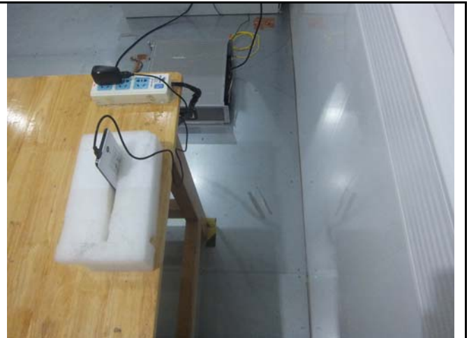
Conducted Emissions Test Setup Side View
