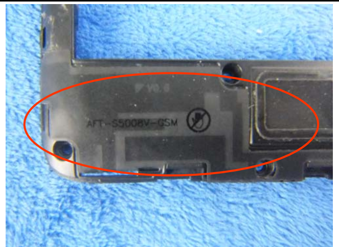
GSM/PCS/UMTS-FDD Antenna View
