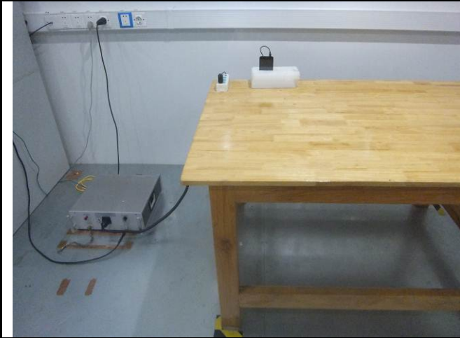
Conducted Emissions Test Setup Front View
