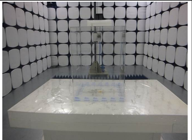
Radiated Spurious Emissions Test Setup Above 1GHz
