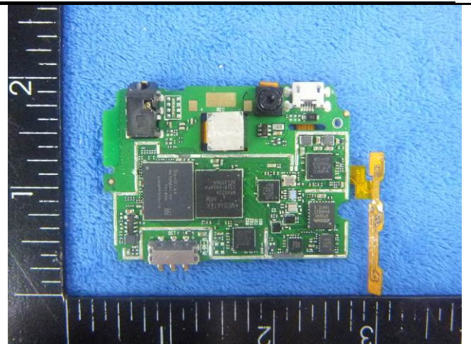
Mainboard Without Shielding - Front View
