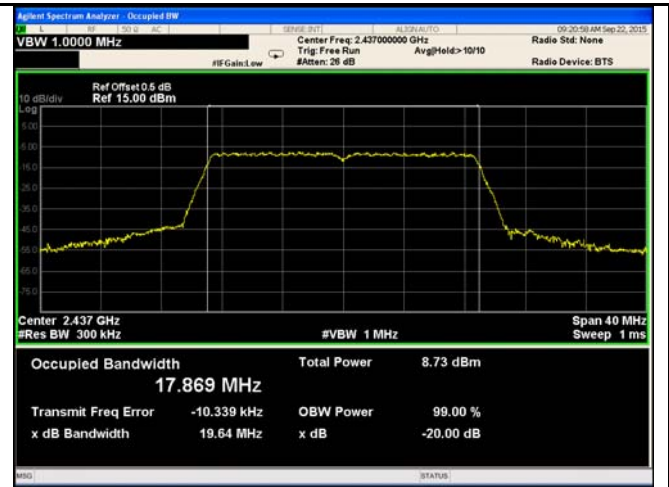
802.11n20 20dB Bandwidth - Mid CH 2437
