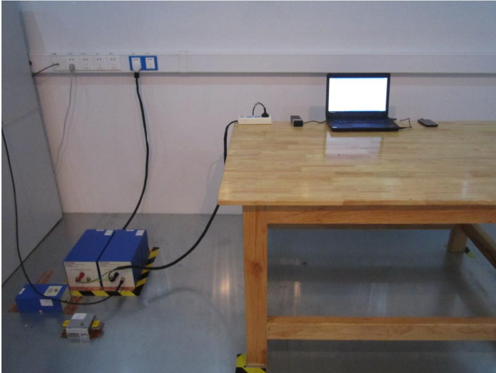
Conducted Emissions Test Setup Front View
