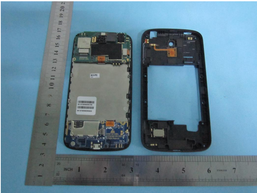
Cover Off - Rear Housing View
