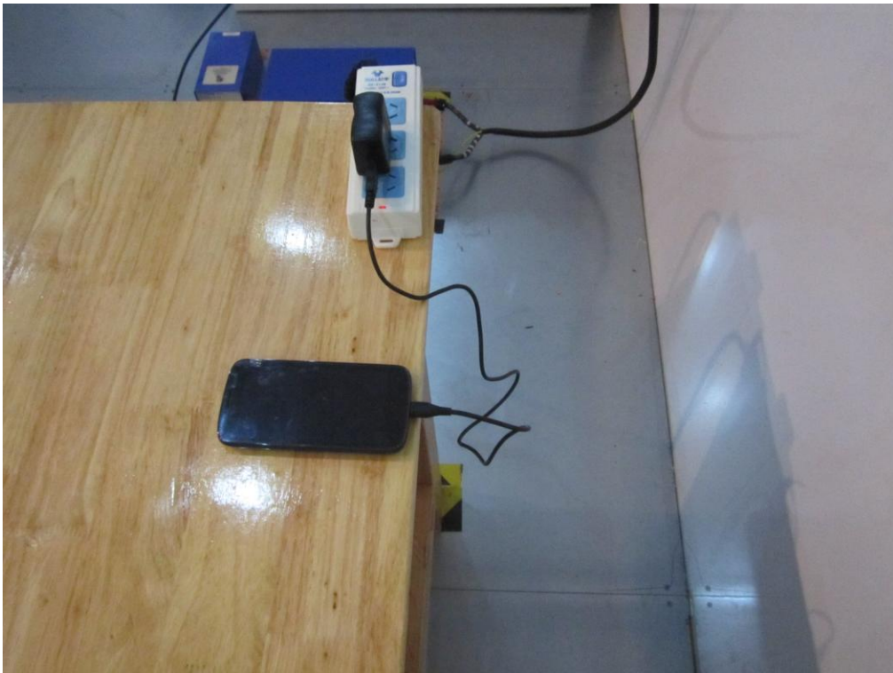
Conducted Emissions Test Setup Side View
