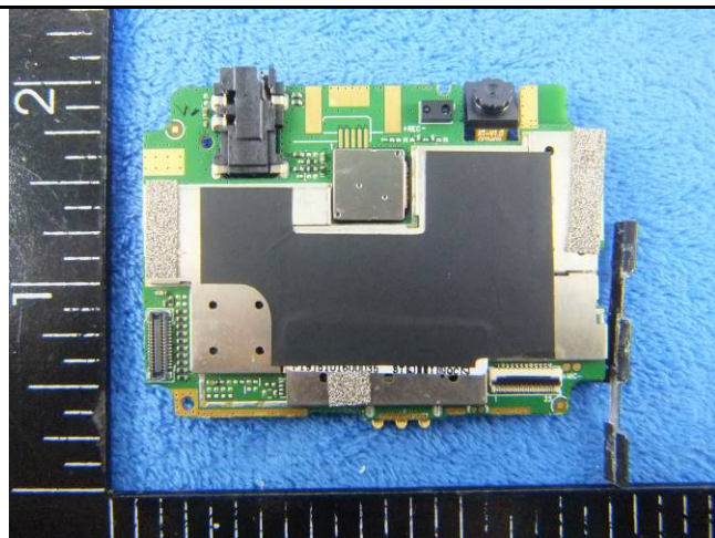
Mainboard With Shielding - Front View
