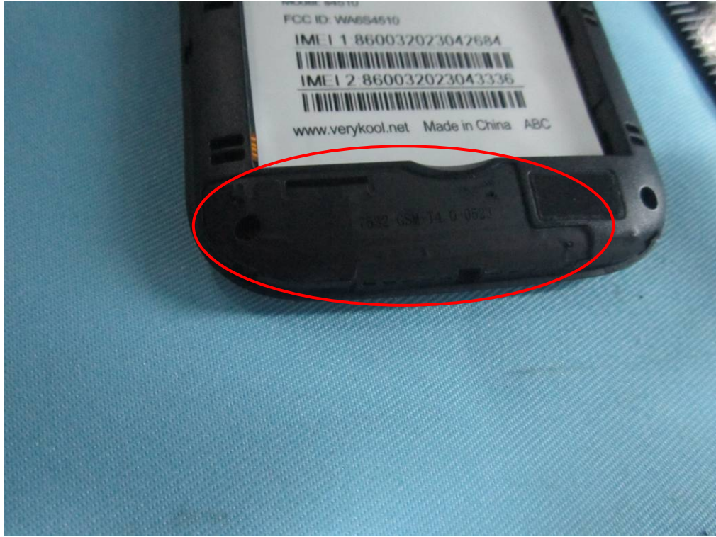
GSM/PCS/UMTS-FDD Antenna View
