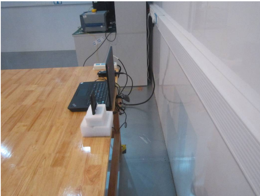
Conducted Emissions Test Setup Side View
