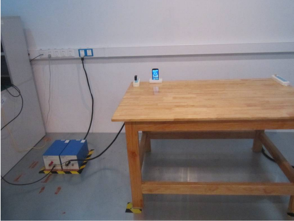
Conducted Emissions Test Setup Front View
