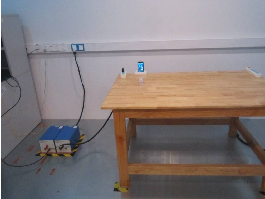
Conducted Emissions Test Setup Front View
