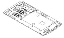
4. Insert the battery by aligning the gold contacts on the battery with the gold contacts in the battery compartment. Gently push down on the battery until it clicks into place.
