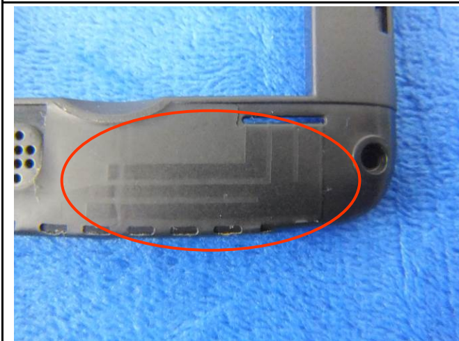
GSM/PCS/UMTS-FDD Antenna View
