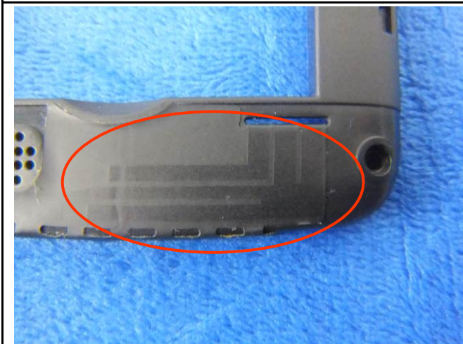
GSM/PCS/UMTS-FDD Antenna View
