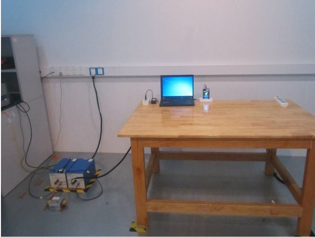
Conducted Emissions Test Setup Front View
