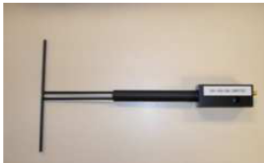
Figure 1 – Satimo COMOSAR Validation Dipole
