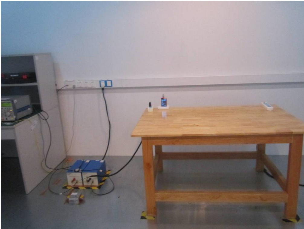
Conducted Emissions Test Setup Front View
