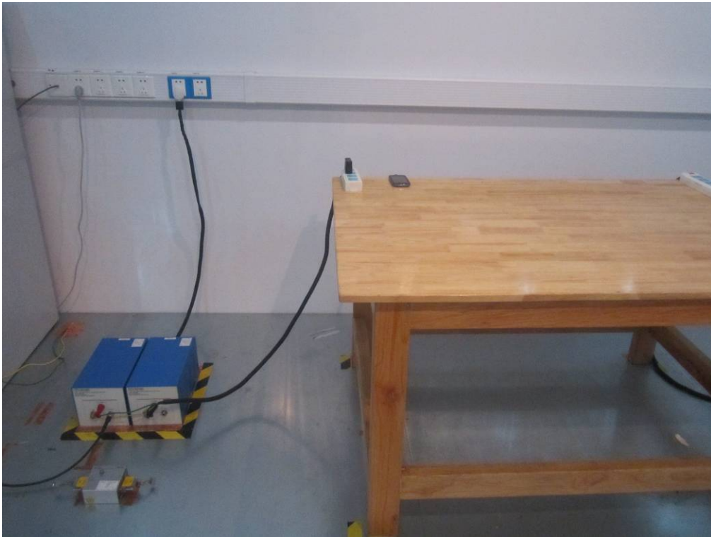
Conducted Emissions Test Setup Front View
