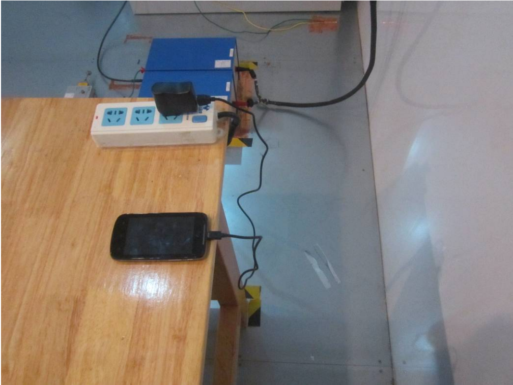
Conducted Emissions Test Setup Side View
